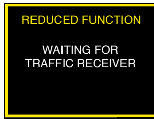
Figure 1.10.: After ATD has been switched on, this screen is shown until data from a connected traffic receiver is available
