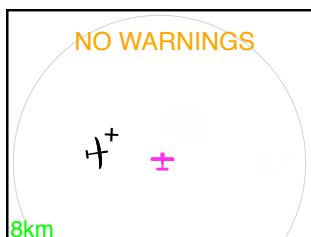
Figure 4.9.: "NO WARNINGS" message appears for the time, warnings are suppressed.
