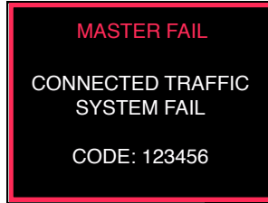
Figure 7.5.: Failure in connected traffic system is detected.
