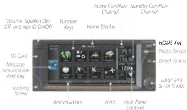
Figure 2 - GTN 635/650 Control and Display Layout
